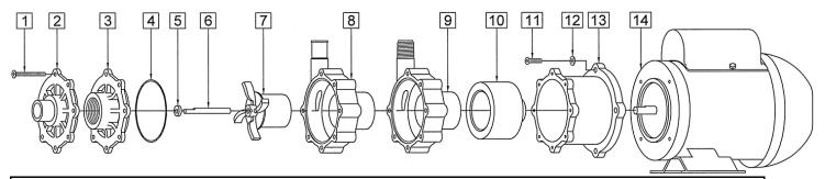
NOTE: When attaching the Drive Magnet to the motor shaft, position the face of the Drive Magnet 3/32 inch below the face of the Motor Bracket.
