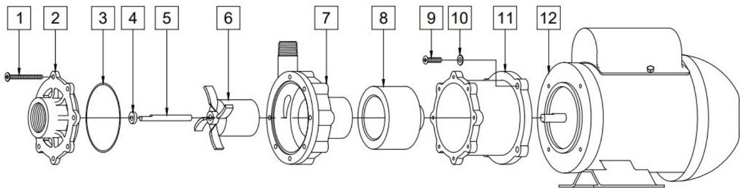
**NOTE:** When attaching the Drive Magnet to the motor shaft, position the face of the Drive Magnet 3/32 inch below the face of the Motor Bracket.
