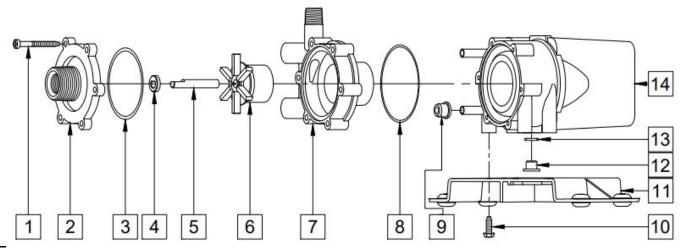
**NOTE:** When attaching the Drive Magnet to the motor shaft, position the face of the Drive Magnet 1/16 inch below the face of the Motor Bracket.
