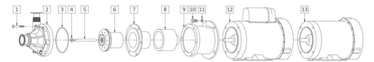
**NOTE:** When attaching drive magnet to the motor shaft, position the face of the drive magnet 1/8 inch below the face of the motor bracket.
