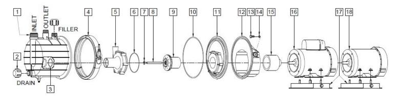
**NOTE:** When replacing impeller bushing in the field: The plastic bushing must be bored to size after they have been pressed into the impeller. Bore to 0.378/0.381 I.D. The carbon and ceramic bushings are to finished size and do not require boring. When attaching drive magnet to the motor shaft, position the face of the drive magnet 49/64 inch above the face of the motor bracket. When reassembling "V" retainer clamp, tighten down to 100-inch pounds.
