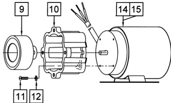
**NOTE:** When attaching the Drive Magnet to the motor shaft, position the face of the Drive Magnet 3/32 inch below the face of the Motor Bracket.
