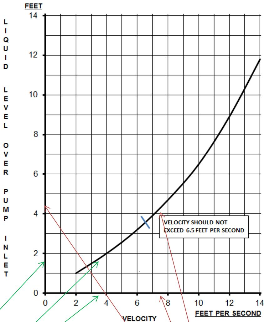
At 3.71 feet per second velocity, the liquid level over the pump must be at minimum 1.8 feet.
